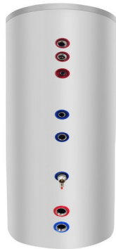
Pressurized Water Tank Model: MWT-200 Capacity: 150+30Liter Max. working pressure: 8 bar Max. hot water temp: 85°C Coil heat exchanger: SUS316L Coil diameter: 25mm Coil length: 15m
